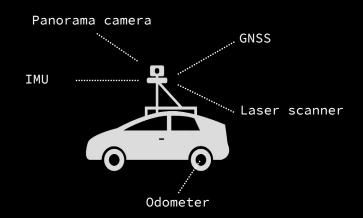
Terrestrial scanning via vehicle-mounted LiDAR technology delivers high-precision 3D data for mapping and modeling. Mounted on vehicles, LiDAR sensors rapidly capture detailed information of the environment, offering a comprehensive solution for urban planning, infrastructure development, and immersive digital replication.
