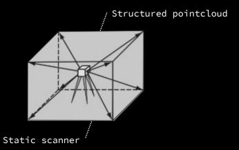
TLS (Terrestrial Laser Scanning) for indoor environments employs laser technology to meticulously capture detailed 3D data. This precise scanning method is ideal for creating digital replicas of indoor spaces, enabling applications in architecture, facility management, and virtual simulations
